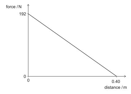
The work done by the force of the bowstring is given by the area under the force-distance graph.
